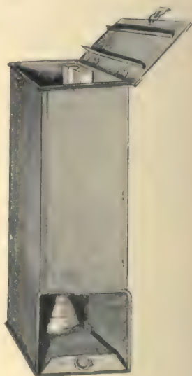
Fig. 184. Drying oven for dragonflies, to take 14 inch setting-boards ( \times \frac{3}{4} ). Original drawing by P. Tillyard.
