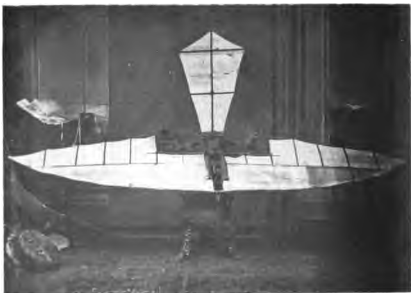
Stringfellow's power-driven model—the first model to achieve engine-driven flight.
