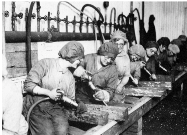
Women workers in ordnance shops, Midval Steel and Ordnance Co., Nicetown, Pa. Hand chipping with pneumatic hammers. 1918. Lt. Lubbe. Credit: National Archives and Records Administration
