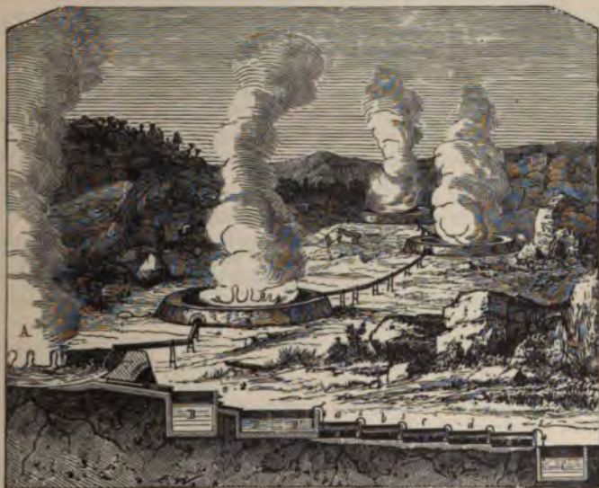
FIG. 81.—Extraction of boric acid in Tuscany.
