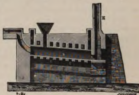
FIG. 85.—Furnace used for the extraction of bismuth from its ores.
