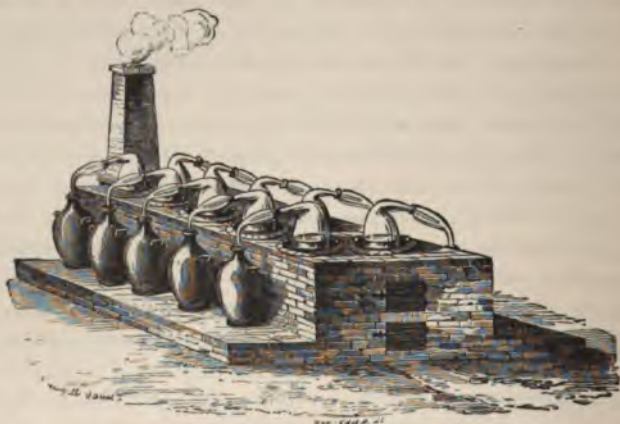
FIG. 87.—Concentration of sulphuric acid in glass retorts. The neck of each retort is attached to a bent glass tube, whose vertical arm is lowered into a glass or earthenware vessel acting as a receiver for the steam which comes over from the acid, as the former still contains a certain amount of acid.
