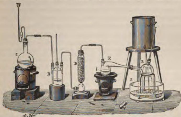
FIG. 91.—Apparatus for the preparation of sulphur chloride, and similar volatile compounds prepared by combustion in a stream of chlorine.
